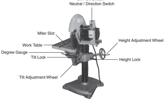
Note: There must be a 1/16" clearance between the Work Table and the face of the Sanding Disc. Refer to Figure 1 above.
